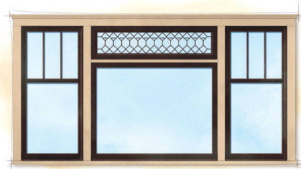
Casement, picture and transom window combination (exterior)
