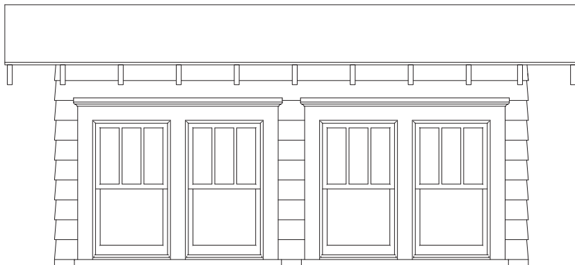
Wide shed dormer with multiple two-wide double-hung window groupings. Typical dormer windows measure between 3' and 4' in height.
