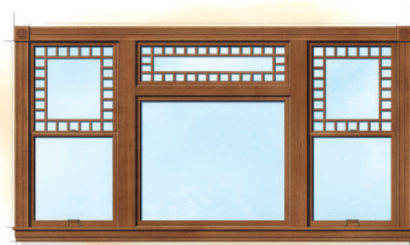
Double-hung, picture and transom window combination (interior)
